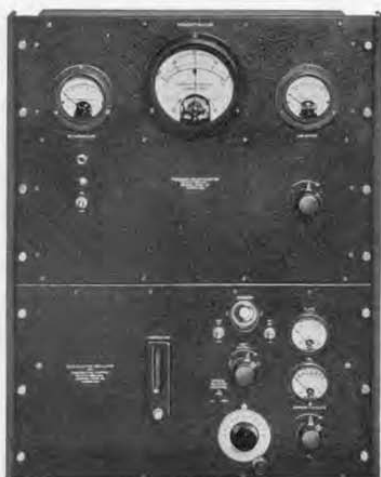
The General Radio Frequency Monitor shown mounted on a desk-type relay rack. Its exceptional performance is due to the use of the new crystal circuit
